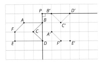
A reflection can be described by a line of reflection (the "mirror"). Each point is reflected directly across the line so that it is just as far from the mirror line, but is on the opposite side.
